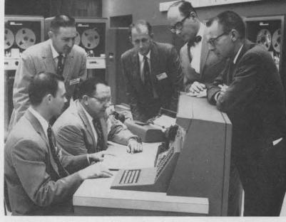
CONTROL CONSOLE of the 705 is studied by Sandia EDPM specialists. The console permits the operator to supervise 705 functions.
